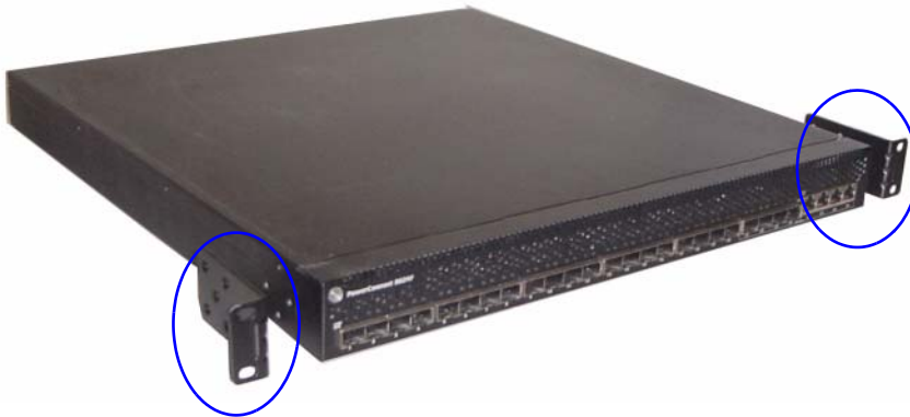
Figure 1. Fixation des supports
