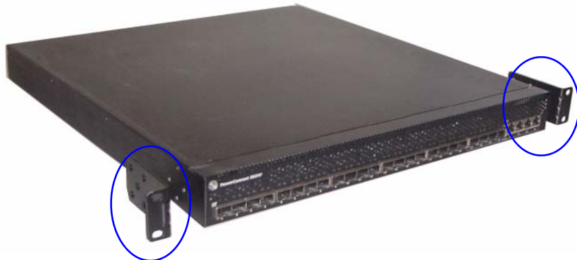
Figure 1. Attaching the Brackets
